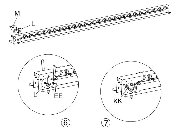
Insert the screwdriver through the hole in the lower part of the louvre mechanism (Part L & M) and rotate the arm to an upright position.
