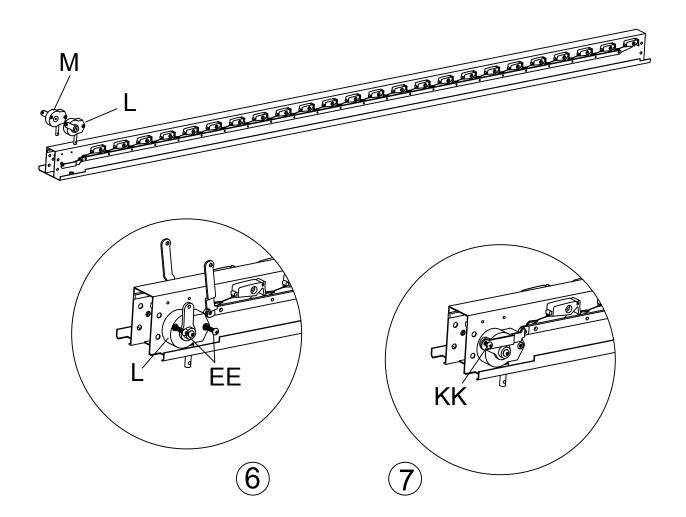
Rotate the lower rod of the turbine can adjust the direction of the steel plate
