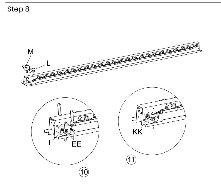
Insert the screwdriver through the hole in the lower part of the mechanism and rotate the arm to an upright position.
