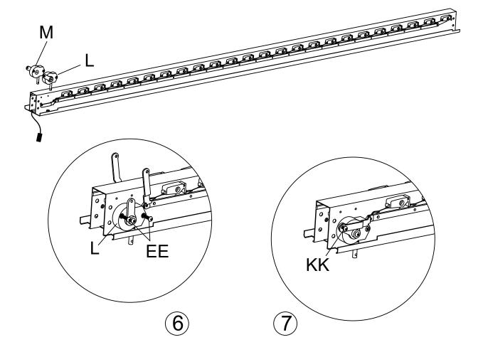
Insert the screwdriver through the hole in the lower part of the mechanism and rotate the arm to an upright position.
